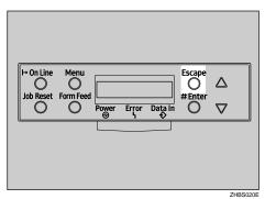
☐ After making the printer settings, press the **[On Line]** key to return to the "Ready" condition.
